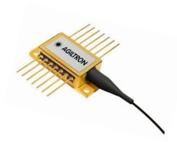
The 1490nm series laser diodes are fabricated in a hermetically sealed 14-pin butterfly package. The laser diodes contain a monitor photodiode, thermoelectric cooler (TEC), and a thermistor to secure high-quality laser performance. Our laser products are Telcordia GR-468 qualified and in compliance with RoHS Directives.
